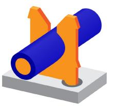
Figure 2 Insulation Displacement Connection [AVX.com]
