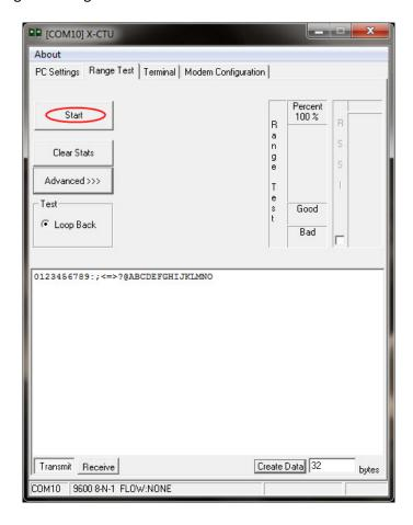
13. Monitor the link quality by reading the Percent section on the Range Test tab. This section displays the running percentage of good packets sent to the receiving radio and looped back to the base.
