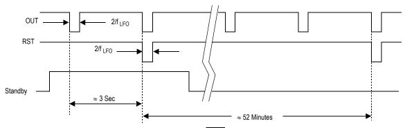
Figure 4. Pulse on RST Pin
