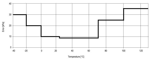
Figure 11. Pressure Error vs Temperature at  $V_{DD}$  = 3.0 V, 250 kPa  $\leq P \leq 450$  kPa
