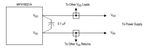
Figure 2. Recommended Power Supply Connections
