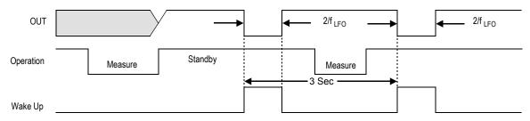
Figure 3. Pulse on OUT Pin During Standby Mode
