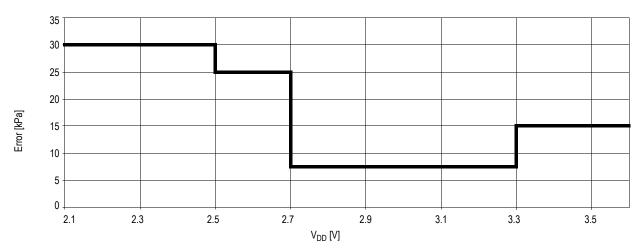
Figure 10. Pressure Error vs  $V_{DD}$  at T = 25°C, 250 kPa  $\leq P \leq$  450 kPa
