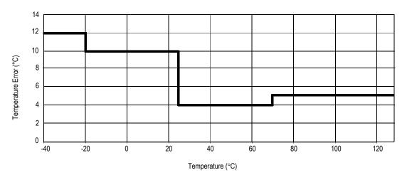
Figure 7. Temperature Error vs Temperature at  $V_{\rm DD}$  = 3.0 V
