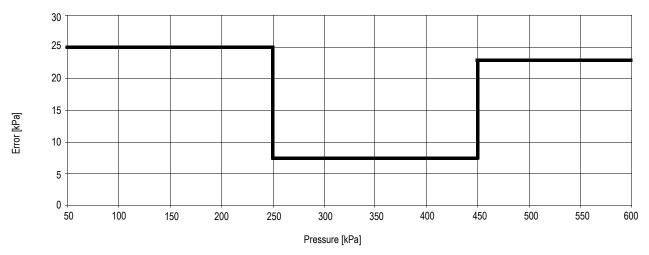
Figure 9. Pressure Error vs Pressure at T = 25°C, 2.7 V  $\leq$  V  $_{DD} \leq$  3.3 V
