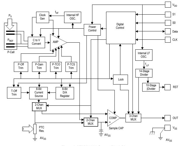
Figure 1. MPXY8021A Sensor Block Diagram
