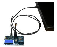
Connect the Programming Docks to a computer with the cables included with the kit. USB drivers are on the CD so install them if prompted by the computer.
