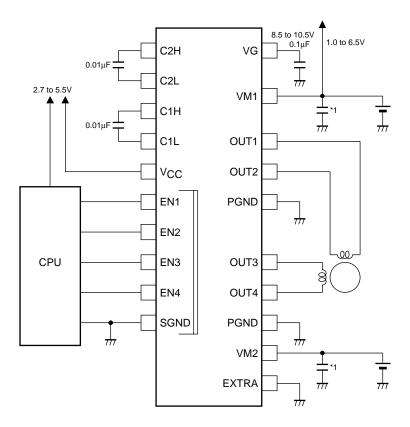
\*1: Connect a kickback absorption capacitor directly near IC. Coil kickback may cause rise of the voltage of VM line, and the voltage exceeding the maximum rating may be applied momentarily, resulting in deterioration or damage of IC.
