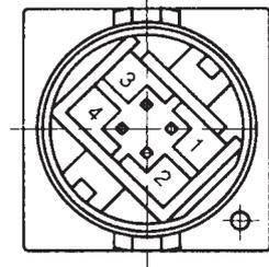
1 + 4 = pushbutton connection, 2 + 3 = lamp connection
