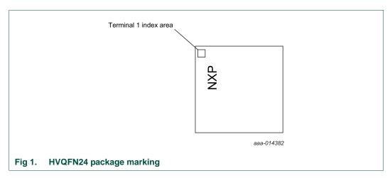
The LPC8N04 HVQFN24 package has the following top-side marking:
