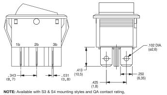
NOTE: Available with S1 & S2 mounting style and Q contact rating only. Shown in Pos. 1
