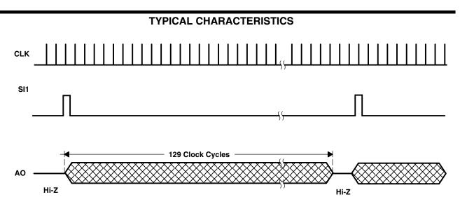
Figure 1. Timing Waveforms (each section)
