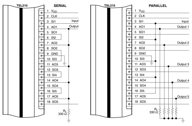
Figure 4. Connection Diagrams
