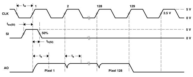
Figure 2. Operational Waveforms (each section)
