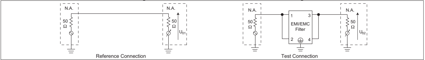
Fig.3.2 Common mode attenuation measurement diagram
