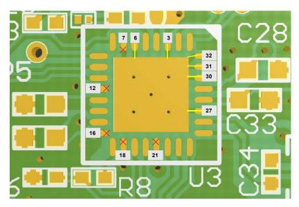
Each ground pin should be connected to the bottom plane with at least one via. Move the vias as close to the IC as possible. It is always desired to integrate the single-pin ground connections into polygon structures after a short distance. Top, bottom, and, on multilayer boards, the inner ground planes, should be tied together with a grid of vias. When ground loops are smaller than one tenth of the wavelength, it is safe to consider this as a solid piece of metal.
