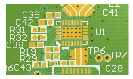
The SE2431L (U1) and associated circuitry follow a standard Skyworks Solutions recommended layout to achieve specified RF performance. The SE2431L requires a central PCB ground pad which is completely relieved of solder resist and has a grid of 15 ground vias [9]. This is essential to achieve good RF performance and adequate thermal conduction, especially in transmit mode. The solder paste mask has limited coverage for assembly purposes.
