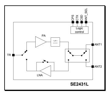
In transmit mode, nominal antenna port transmit output power is +20dBm for Atmel AT86RF231 sub-register setting TX\_PWR = 0x0A at EVDD = 3.0V nominal supply voltage. Second and third harmonics levels are less than - 42dBm/MHz. Transmit output power level is adjusted using the AT86RF231 TX output power, controlled via register bits TX\_PWR.
