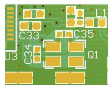
When designing applications for very harsh environments, for example where the radio transceiver is close to mains power lines and burst and surge requirements already dictate special provisions in the design, the above reference crystal design might not work well. In this case, the reference crystal ground is to be directly connected to top and bottom layers.
