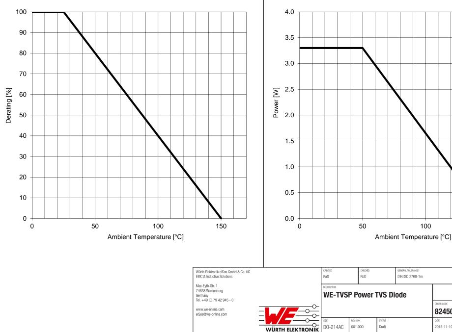
**Steady State Power Dissipation Derating**
