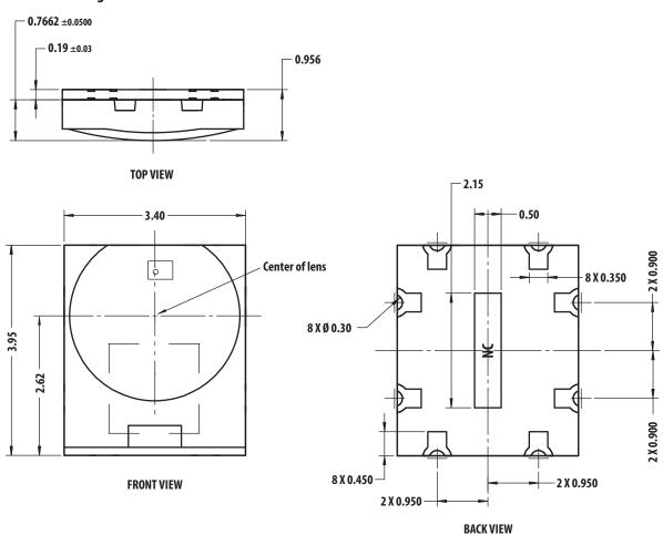
\* All dimensions in millimeter. Tolerance x.xx  $\pm$  0.15 mm
