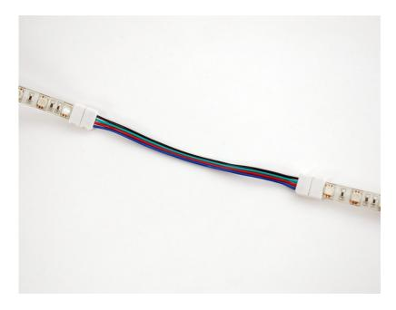
Close the plastic covers and you're done! Pictured here is the extender cable with strips attached on either end.
