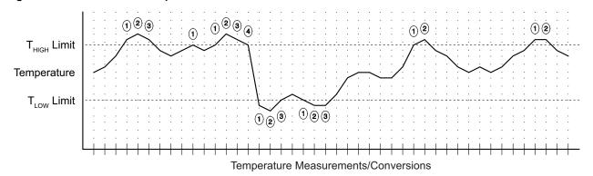
Figure 5-1. Fault Count Example
