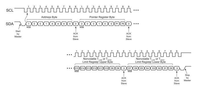
Figure 6-11. Read to Nonvolatile T<sub>LOW</sub> or T<sub>HIGH</sub> Limit Register
