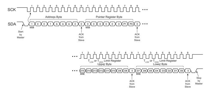
Figure 6-9. Read from T<sub>LOW</sub> or T<sub>HIGH</sub> Limit Register
