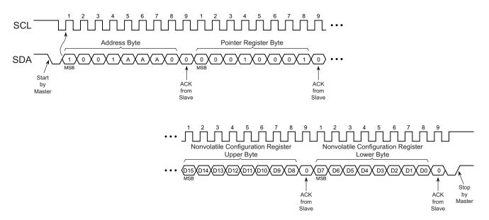
Figure 6-7. Read from Nonvolatile Configuration Register
