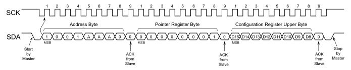
Figure 6-5. Read from Configuration Register
