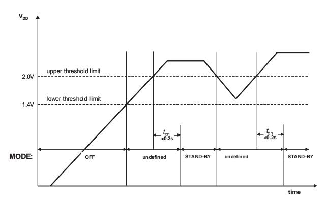
The threshold limit where the device switches from OFF to STAND-BY is between  $V_{\rm DD}$  =1.4V and  $V_{\rm DD}$  =2.0V. Within 0.2s after exceeding the threshold voltage the device will switch from OFF to STAND-BY mode.
