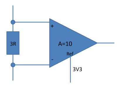
Figure 13: TX current measurement amplifier
