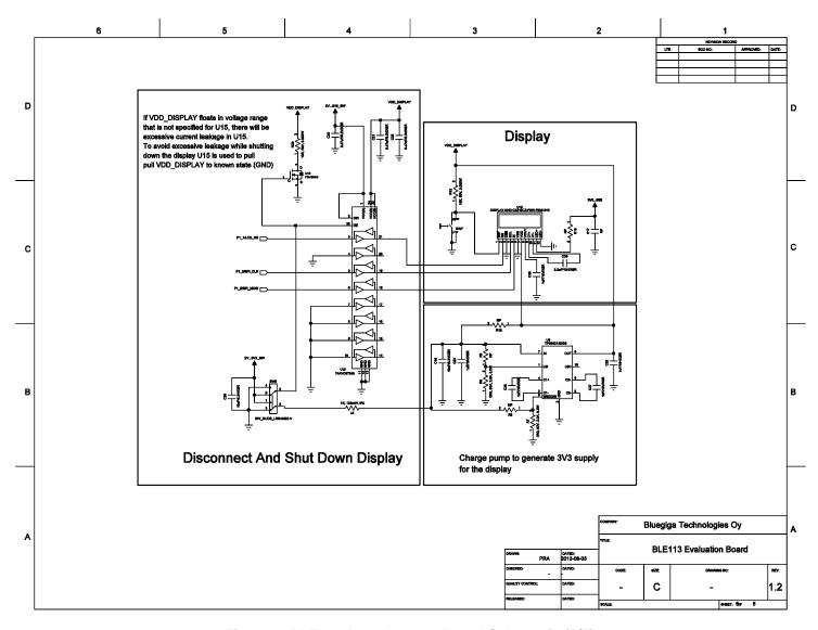
Figure 7: BLE113 Development Board Schematic (5/5)
