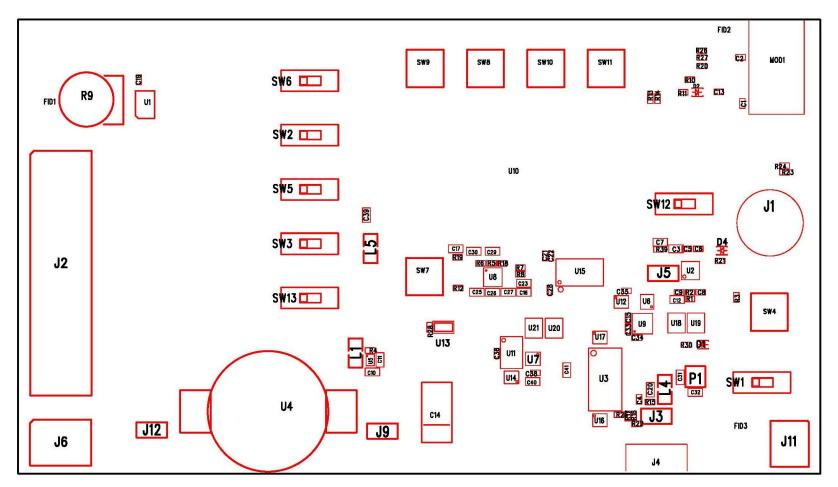
Figure 8: BLE113 Development Board Assembly Drawing
