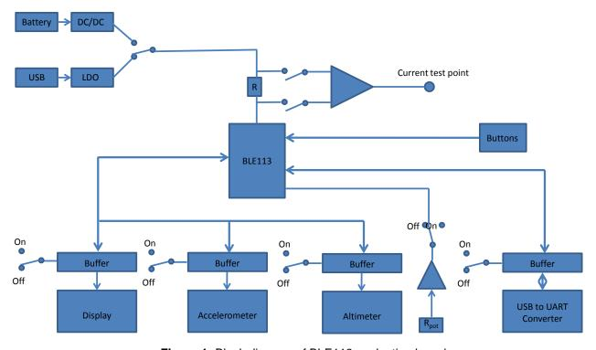
Figure 1: Block diagram of BLE113 evaluation board
