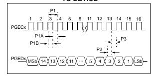
Since a 2-wire SPI is used, and data transmissions are half-duplex, a simple protocol is used to control the direction of PGEDx. When the programmer completes a command transmission, it releases the PGEDx line and allows the Programming Executive to drive this line high. The Programming Executive keeps the PGEDx line high to indicate that it is processing the command.
