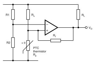
Fig. 1 Typical comparator circuit
