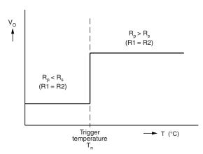
Fig. 2 Typical switch characteristic
