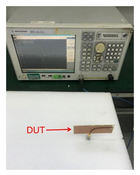
FIGURE4.1.2 ANTENNA LOADED WITH VNA
