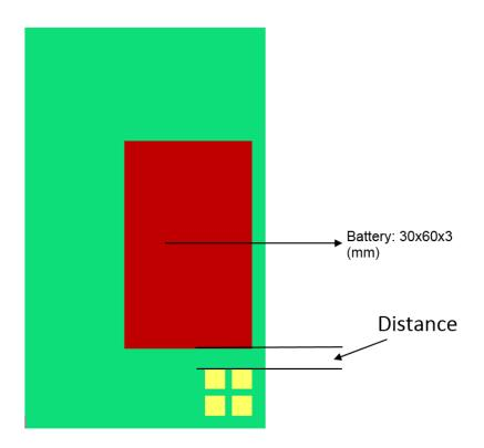
FIGURE 7.2.1 BATTERY FIXED ON REFERENCE PCB
