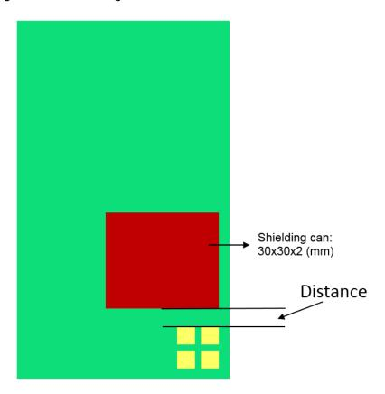
FIGURE 7.1.1 SHIELDING CAN FIXED ON REFERENCE PCB
