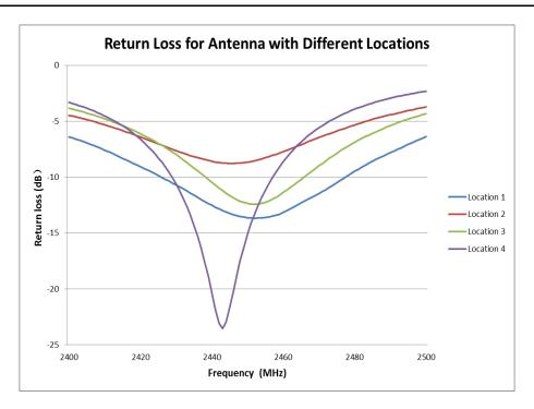
FIGURE 7.3.2 RETURN LOSS COMPARISON AT 2.4 GHZ BAND AT FOUR LOCATIONS
