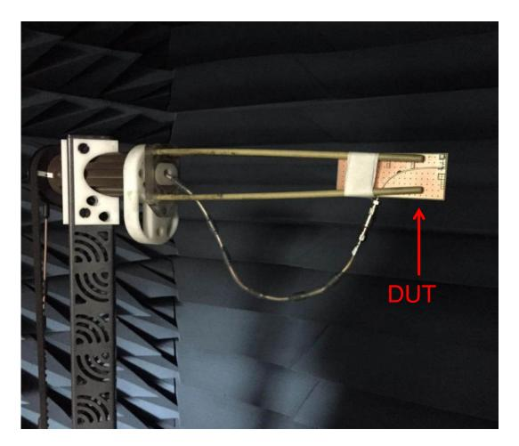
FIGURE4.1.3 ANTENNA LOADED WITH OTA CHAMBER
