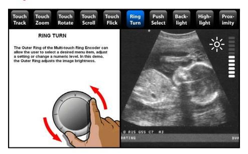
The MTRE touchpad has a unique outer ring that rotates. This ring is perfect for setting machine levels or switching between machine functions. Of course, the actual settings or function that the ring can control can be changed based on the current state of the machine.
