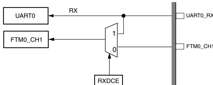
**Figure 3-3. UART0\_RX capture function diagram**
