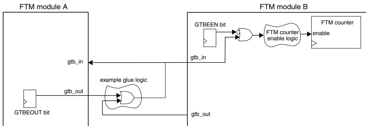
**Figure 26-247. Global time base (GTB) block diagram**
