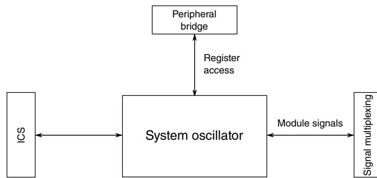
**Figure 3-16. OSC configuration****Table 3-20. Reference links to related information**
