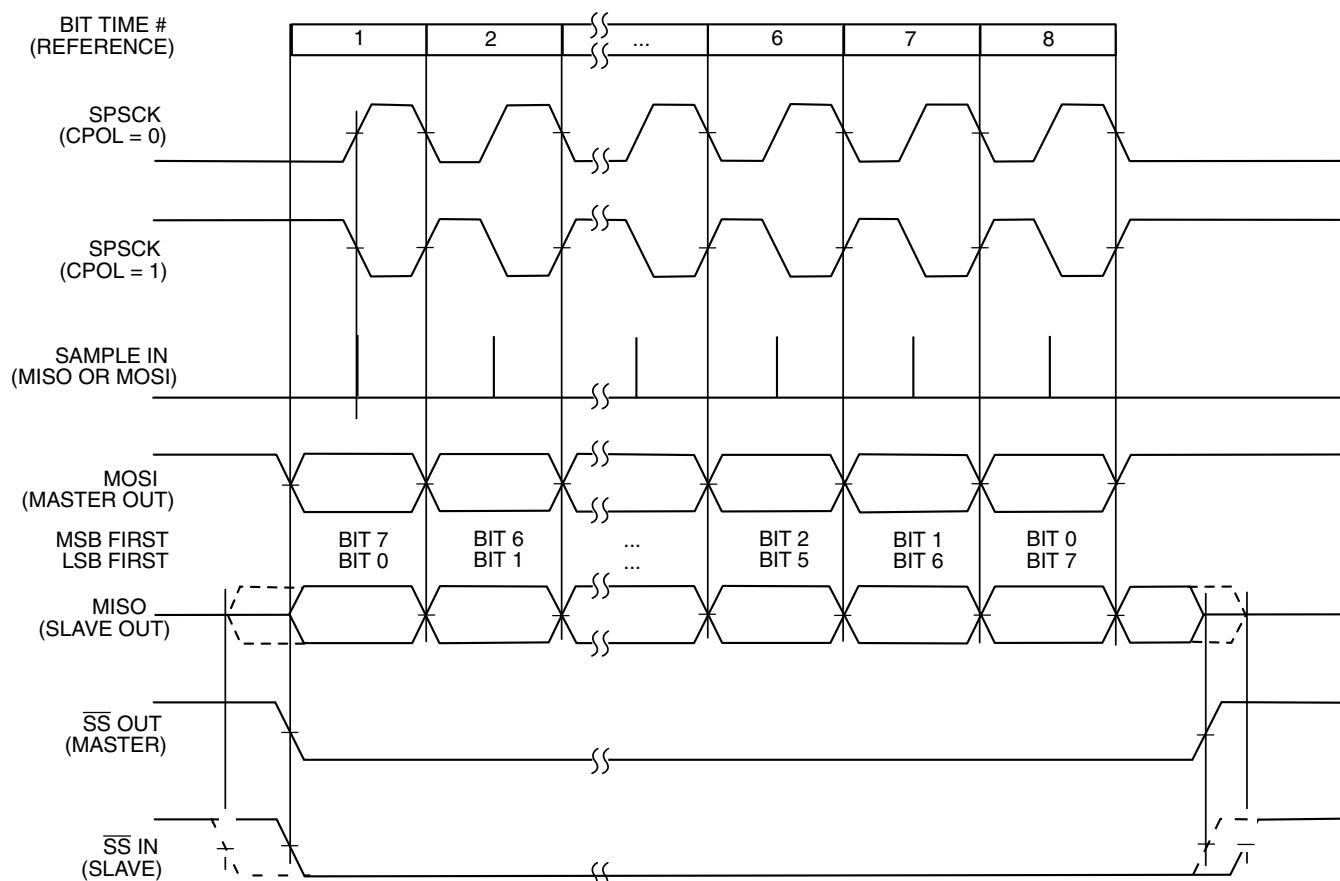
Figure 29-22. SPI clock formats (CPHA = 0)
