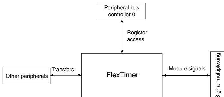
**Figure 3-24. FlexTimer configuration****Table 3-32. Reference links to related information**
