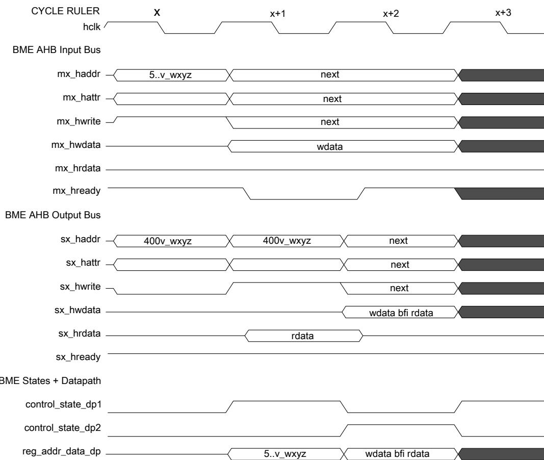
**Figure 17-2. Decorated store: bit field insert timing diagram**
