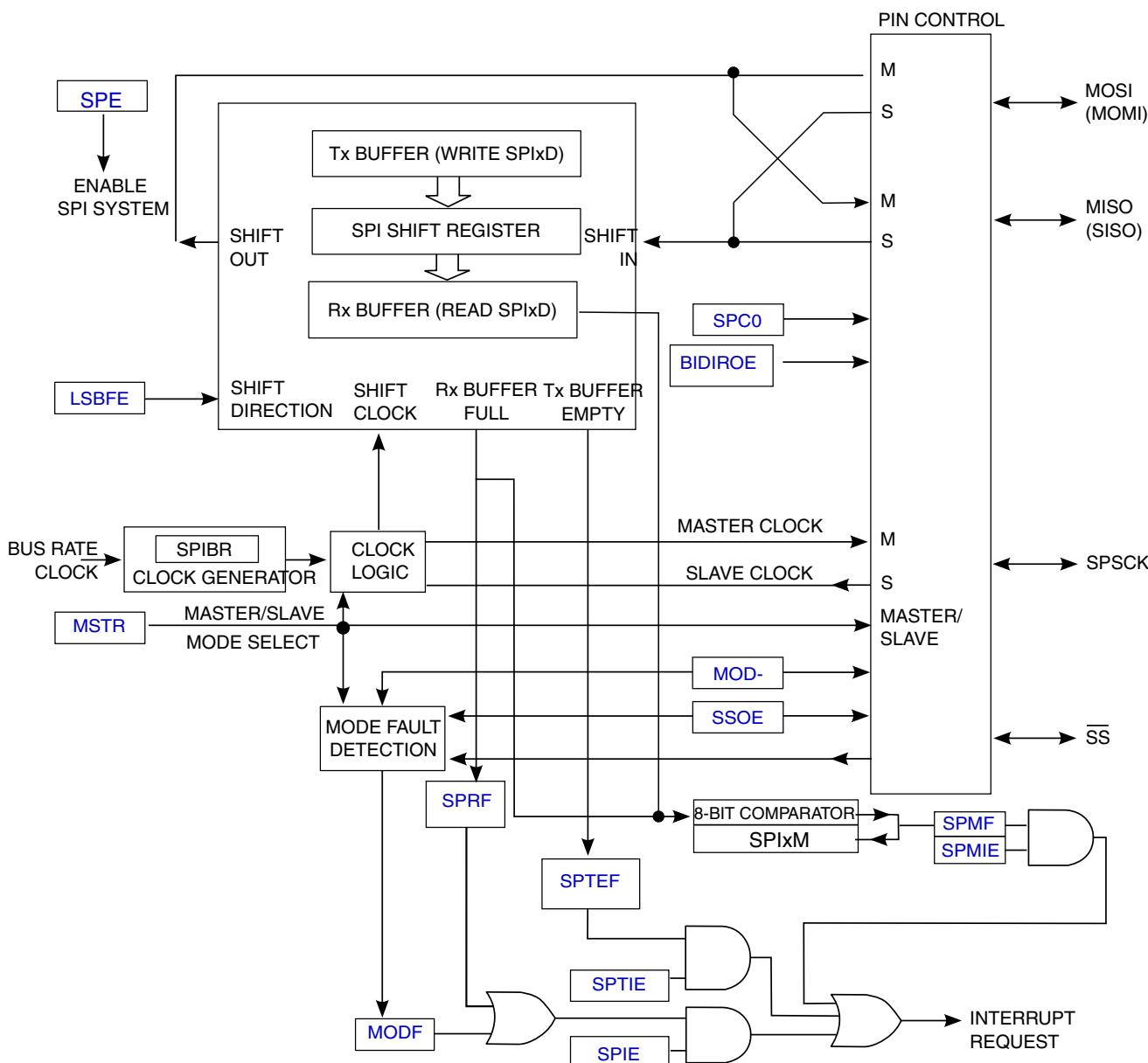
Figure 29-2. SPI module block diagram without FIFO
