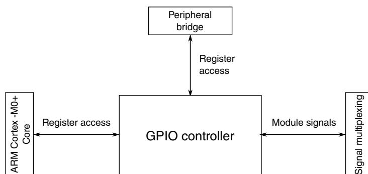
**Figure 3-30. GPIO configuration**
