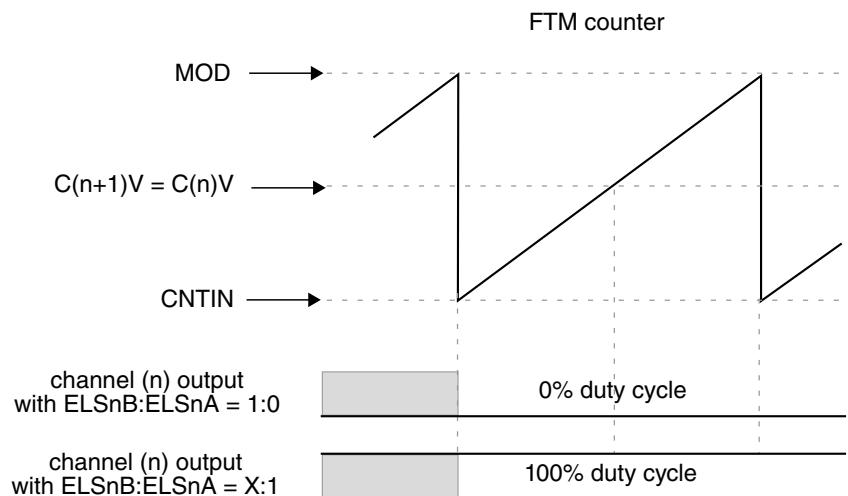
**Figure 26-190. Channel (n) output if ( $C(n)V < C(n+1)V < MOD$ ) and ( $CNTIN < C(n)V < C(n+1)V$ ) and ( $C(n)V = C(n+1)V$ )**
