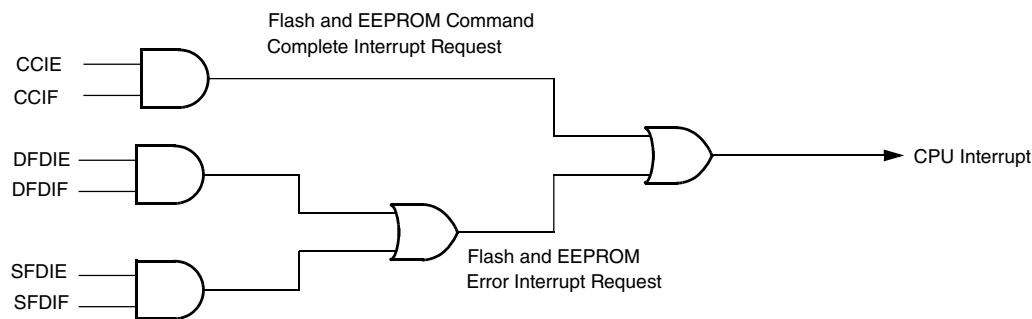
**Figure 18-2. Flash and EEPROM module interrupts implementation**
