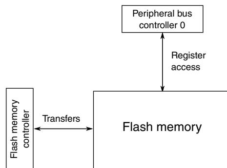
**Figure 3-17. Flash memory configuration****Table 3-21. Reference links to related information**
