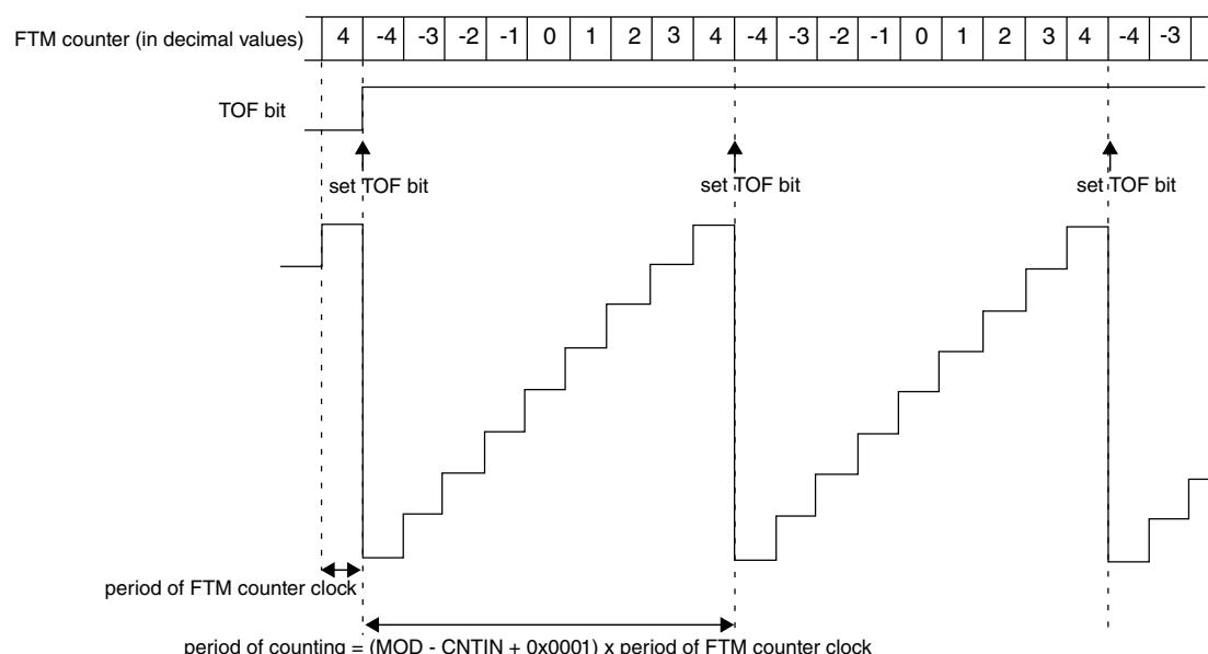
**Figure 26-164. Example of FTM up and signed counting**
