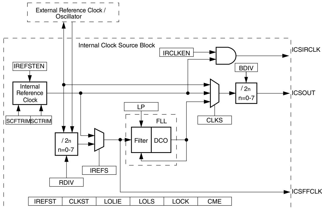
**Figure 20-1. Internal clock source (ICS) block diagram**
