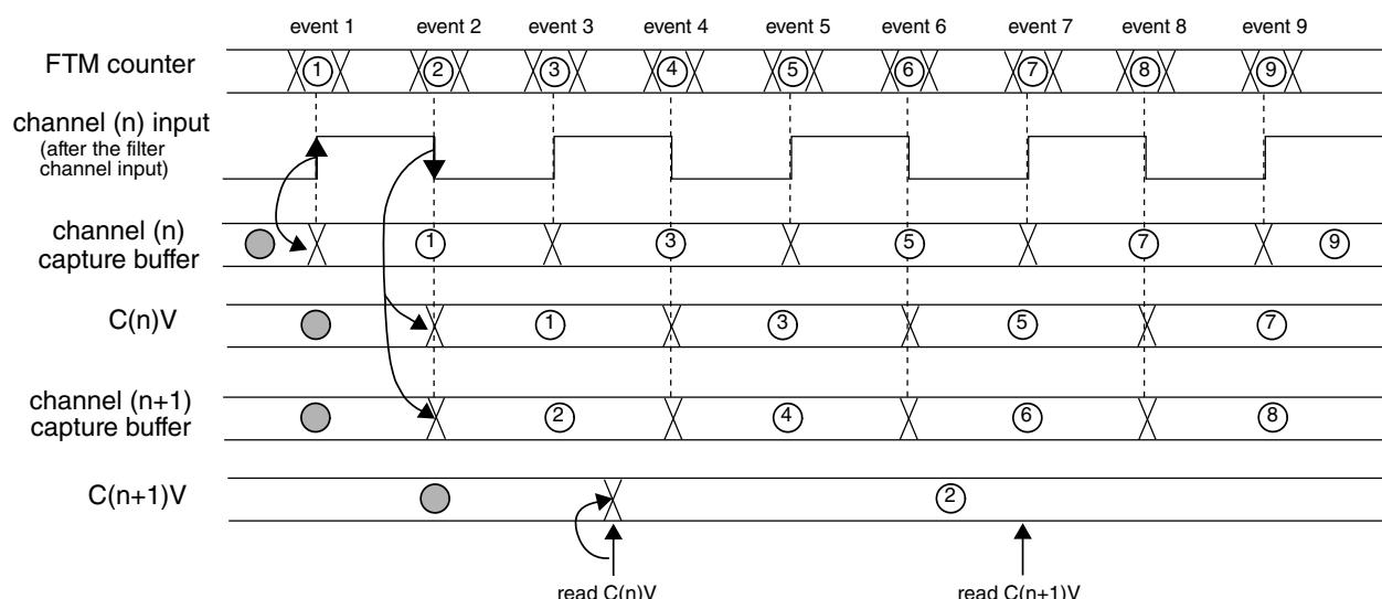
**Figure 26-245. Dual Edge Capture mode read coherency mechanism**
