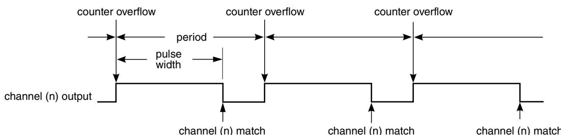
**Figure 26-177. EPWM period and pulse width with ELSnB:ELSnA = 1:0**
