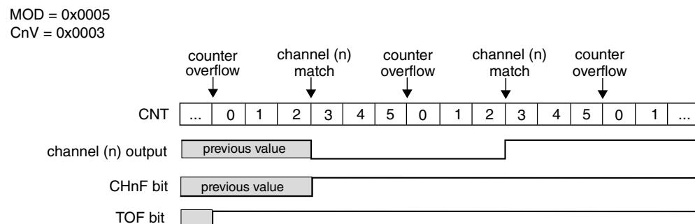
**Figure 26-174. Example of the Output Compare mode when the match toggles the channel output**
