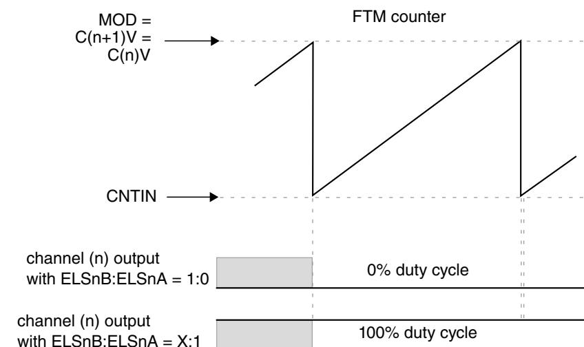
**Figure 26-192. Channel (n) output if ( $C(n)V = C(n+1)V = MOD$ )**
