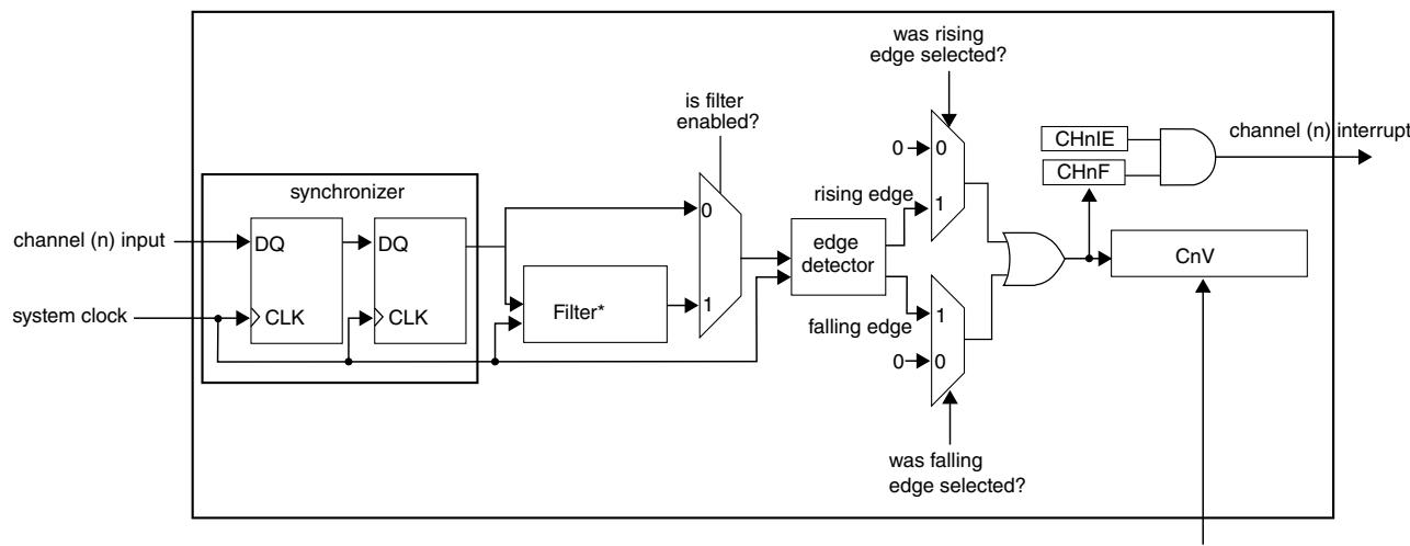
**Figure 26-171. Input Capture mode**
