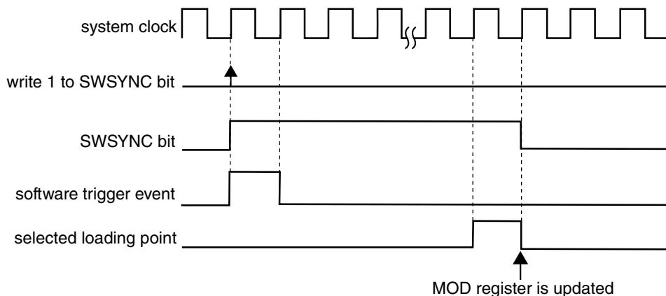
**Figure 26-209. MOD synchronization with (SYNCMODE = 0) and (PWMSYNC = 1)**
