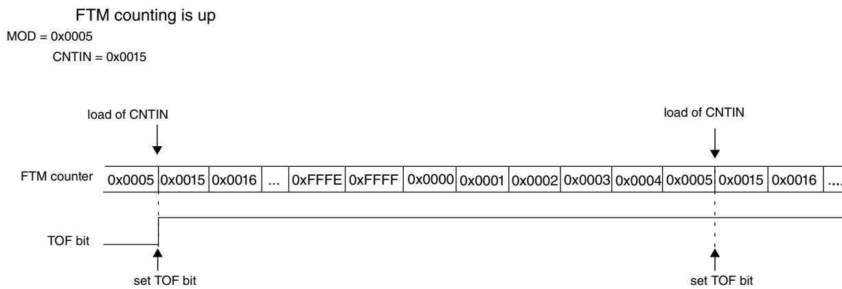
**Figure 26-166. Example of up counting when the value of CNTIN is greater than the value of MOD**
