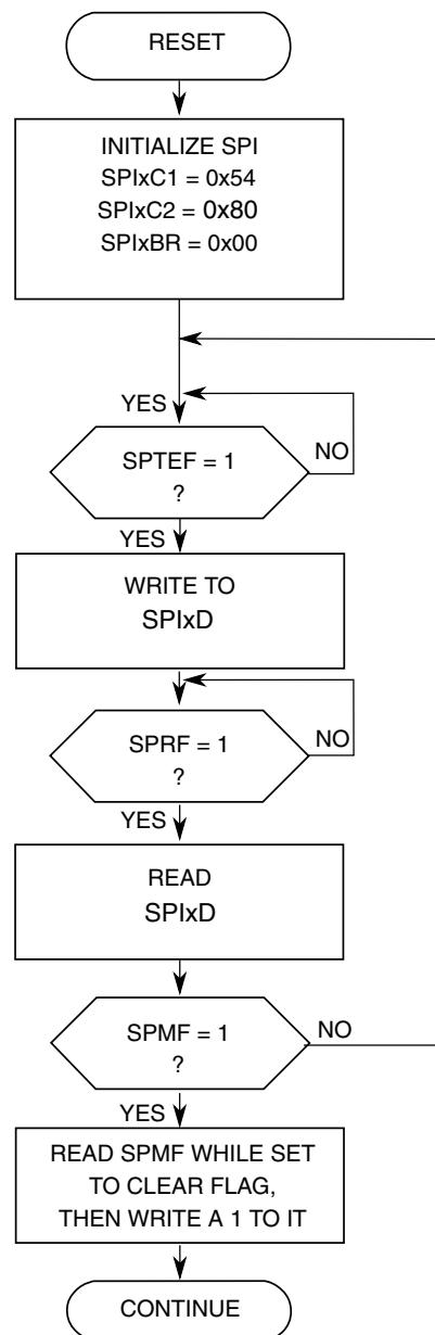
**Figure 29-24. Initialization Flowchart Example for SPI Master Device**
