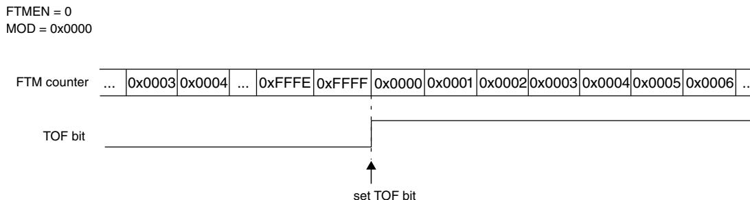
**Figure 26-168. Example when the FTM counter is free running**
