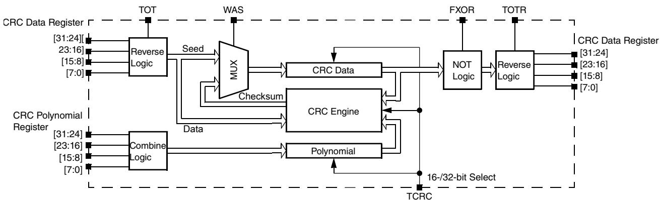
Figure 22-1. Programmable cyclic redundancy check (CRC) block diagram
