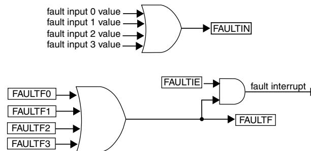
**Figure 26-230. FAULTF and FAULTIN bits and fault interrupt**
