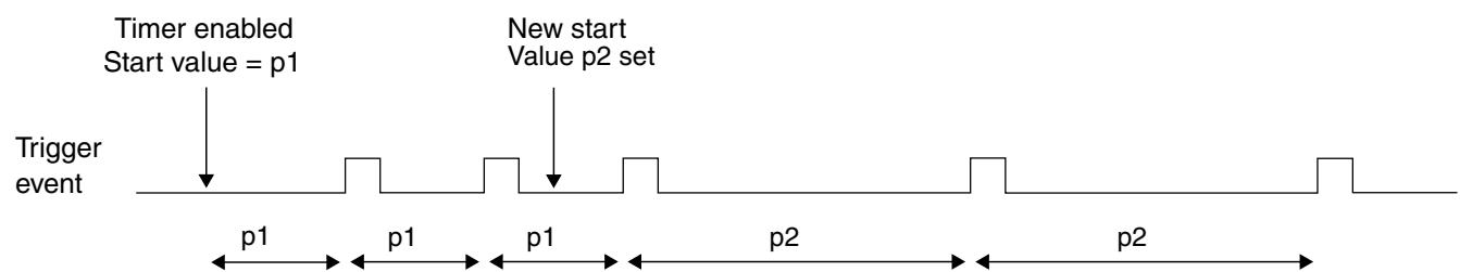
**Figure 27-17. Dynamically setting a new load value**
