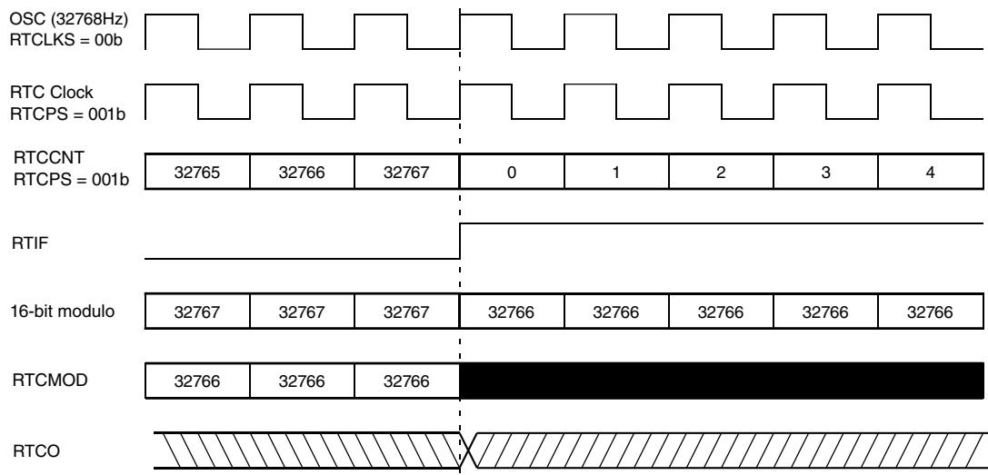
**Figure 28-5. RTC counter overflow example**
