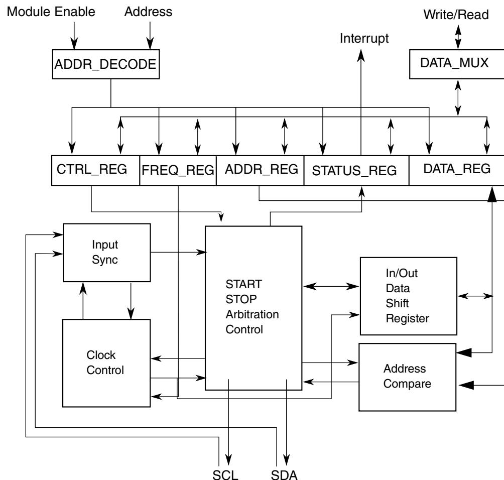
**Figure 30-1. I<sup>2</sup>C Functional block diagram**
