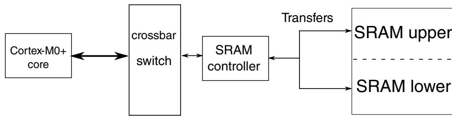
**Figure 3-20. SRAM configuration****Table 3-24. Reference links to related information**
