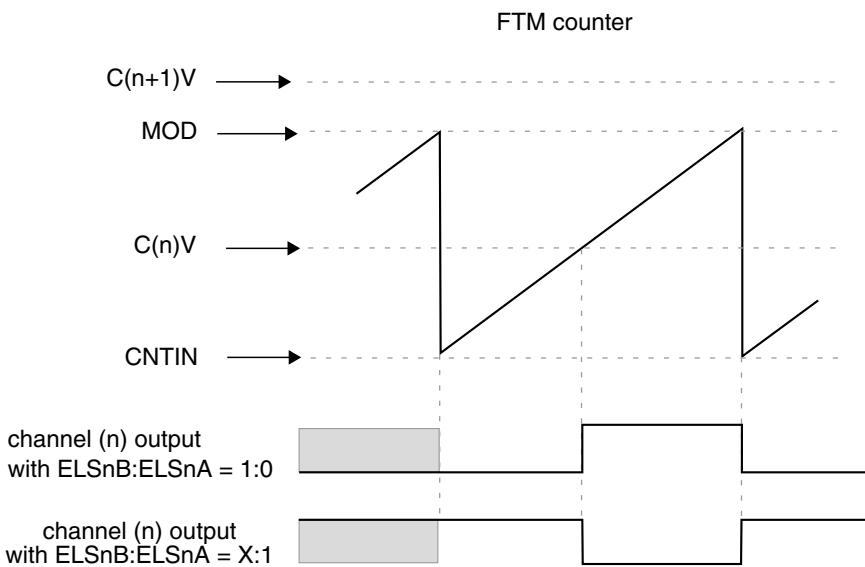
**Figure 26-197. Channel (n) output if ( $C(n+1)V > MOD$ ) and ( $CNTIN < C(n)V < MOD$ )**
