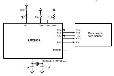
Figure 2. Example For A Cable Replacement Application
