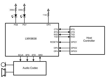
Figure 3. Example For Host Controller Based Application With Audio Support
