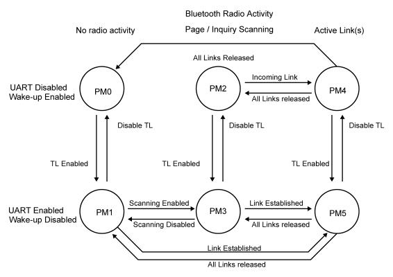
Figure 7. Transition between different Hardware Power Modes
