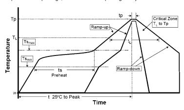
Figure 14. Typical Reflow Profiles
