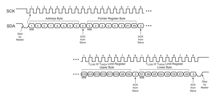
Figure 5-7. Read from T<sub>LOW</sub> or T<sub>HIGH</sub> Limit Register
