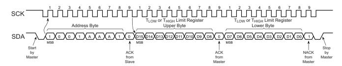
Note: Assumes the Pointer Register was previously set to point to the T<sub>LOW</sub> or T<sub>HIGH</sub> Limit Register.
