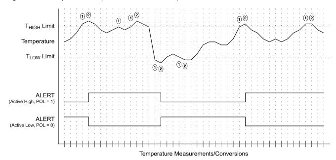
Figure 4-3. Comparator Mode (Fault Tolerance Queue = 2)
