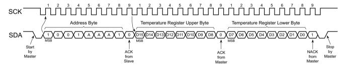
Note: Assumes the Pointer Register was previously set to point to the Temperature Register.
