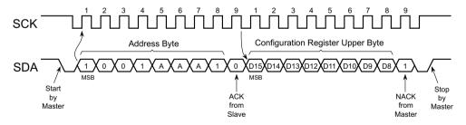
Note: Assumes the Pointer Register was previously set to point to the Configuration Register.
