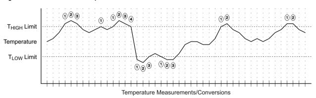
Figure 4-2. Fault Count Example
