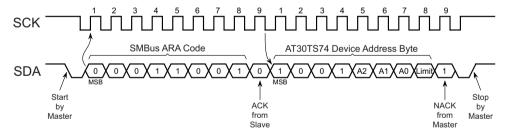
Note: The Limit bit (the LSB) of the device address byte will be one or zero depending on if the T<sub>HIGH</sub> or T<sub>LOW</sub> limit was exceeded.
