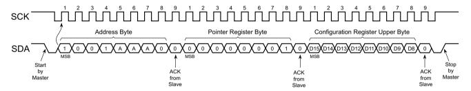
Figure 5-5. Read from Configuration Register
