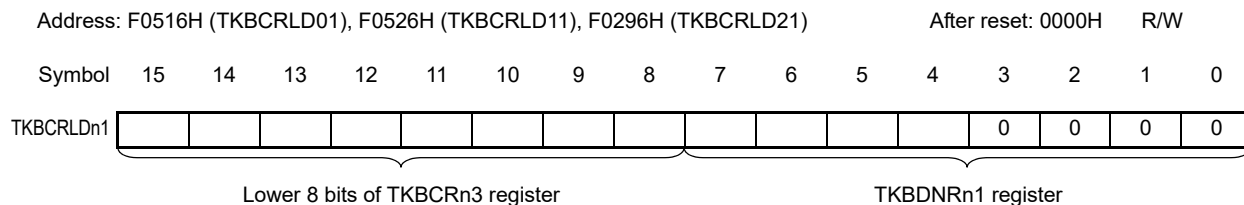
Figure 7 - 19 Format of 16-bit timer KB2 compare 1L & dithering count register n1 (TKBCRLDn1)
