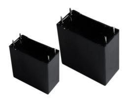
Type 953B radial leaded metallized polypropyene capacitors are designed for UPS systems and other AC output filtering applications. With an integrated fused metallization pattern, this product features UL 810 recognition for fail-safe operation at temperatures up to 85 °C.
