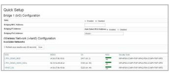
3. In the Quick Setup page, bridging and wireless interfaces can be configured. Bridging can be enabled and the Premierwave 2050 can be connected to a network from the list of available wireless networks.
