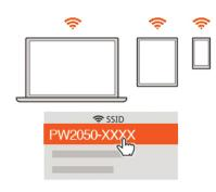
1. Connect to SSID PW2050-XXXX, where XXXX refers to the SN on the evaluation board.
