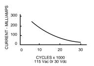
One cycle is  $360^\circ$  rotation clockwise and  $360^\circ$  return. The data for the curve was measured at sea level,  $25^\circ\text{C}$  and 68% relative humidity with the life limiting criteria which follows.
