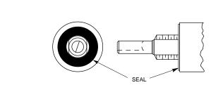
Panel is sealed by an O-ring at the base of bushing. Shaft is sealed by an O-ring inside the bushing. After the switch is mounted, seals do not alter the dimensions of the unsealed style.
