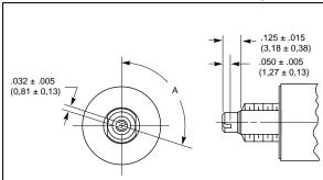
Series 56 rotary switches are available with a screwdriver slotted shaft with dimensions as shown. Available in the styles, angles of throw and pole/positions combinations shown in the choice and limitations chart.
