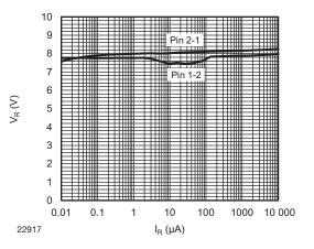
Fig. 6 - Typical Reverse Voltage vs. Reverse Current
