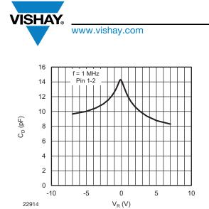
Fig. 3 - Typical Capacitance vs. Reverse Voltage
