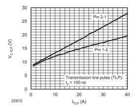
Fig. 4 - Typical Camping Voltage vs. Peak Pulse Current
