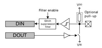
When MODEn=0b0101 or 0b11xx, the output driver uses the drive strength specified in DRIVEMODE in GPIO\_Px\_CTRL. In all other output modes, the drive strength is set to STANDARD.
