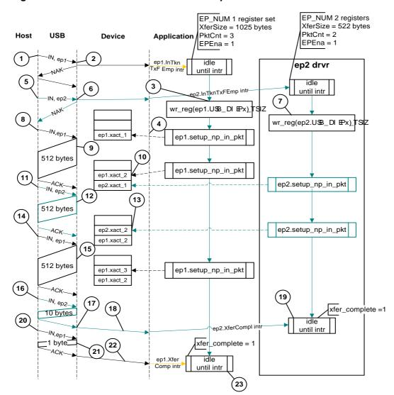
Figure 15.29. Slave Mode Bulk IN Two-Endpoint Transfer
