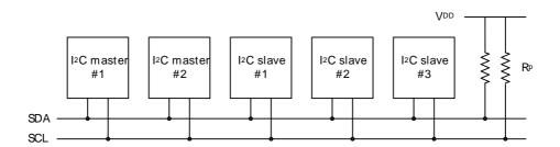
Each device on the bus is addressable by a unique address, and an I<sup>2</sup>C master can address all the devices on the bus, including other masters.
