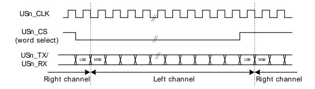
Figure 17.17. USART Standard I2S waveform (reduced accuracy)
