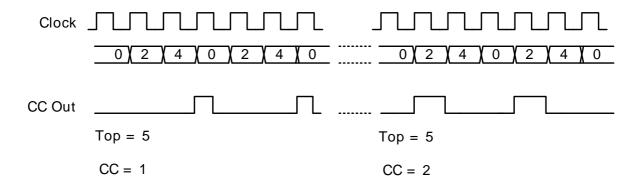
The mode is enabled by setting the X2CNT field in TIMERn\_CTRL register. The intended use of the 2x mode is to generate 2x PWM frequency when the Compare/Capture channel is put in PWM mode. Since the PWM output is updated on both edges of the clock, frequency prescaling will result in incorrect result in this mode. The PWM resolution (in bits) is then given by Equation 20.6 (p. 535).
