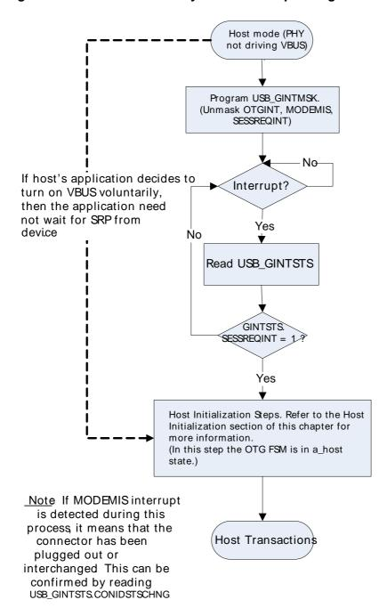
Figure 15.33 (p. 328) illustrates the steps that need to be performed by B-device's application (core as B-device) in order to establishing a connection with A-device by signaling a SRP.
