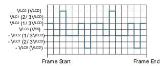
1/3 bias and quadruplex multiplexing - LCD SEG0-LCD COM2
