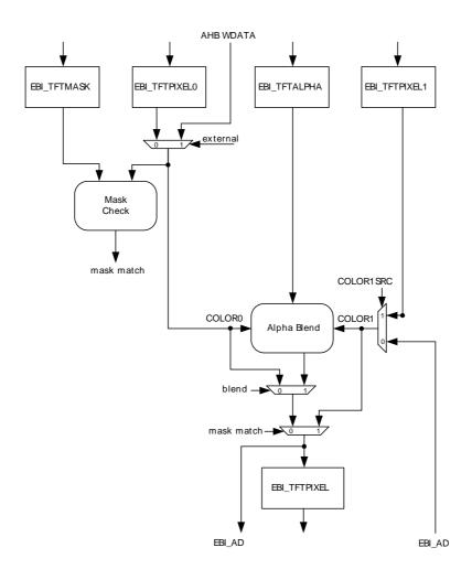
external = (MASKBLEND == BMASK) or (MASKBLEND == EALPHA) or (MASKBLEND == BMASKEALPHA) blend = (MASKBLEND == IALPHA) or (MASKBLEND == EALPHA)
