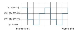
Figure 33.14. LCD 1/3 Bias and Duplex Multiplexing - LCD\_SEG0 Connection
