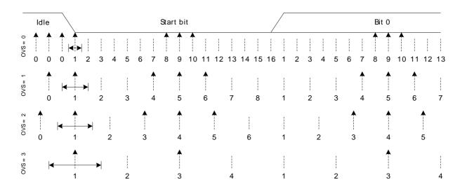
If the baud rate of the transmitter and receiver differ, the location each bit is sampled will be shifted towards the previous or next bit in the frame. This is acceptable for small errors in the baud rate, but for larger errors, it will result in transmission errors.
