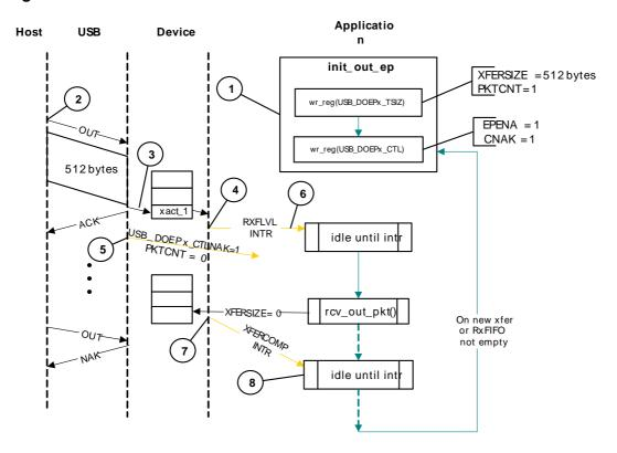
After a SetConfiguration/SetInterface command, the application initializes all OUT endpoints by setting USB\_DOEPx\_CTL.CNAK = 1 and USB\_DOEPx\_CTL.EPENA = 1, and setting a suitable XFERSIZE and PKTCNT in the USB\_DOEPx\_TSIZ register.
