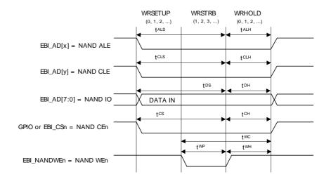
The EBI\_WRTIMING(n) setting requirements for satisfying the NAND Flash timing parameters for command latching, address latching and data input timing are shown in Table 14.5 (p. 195).
