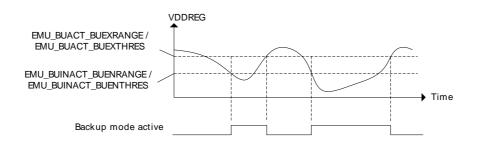
Figure 10.4 (p. 113) illustrates how the BOD sensing on VDD\_DREG can be programmed to implement hysteresis on entering and exiting backup mode.
