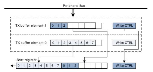
As shown in Figure 17.9 (p. 462), frame transmission control bits are taken from the second element in FIFO.
