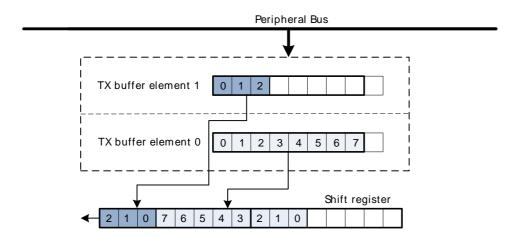
Figure 17.10 (p. 462) illustrates the order of the transmitted bits when an 11 bit frame is transmitted with MSBF set. If MSBF is set and the frame is smaller than 10 bits, only the contents of transmit buffer 0 will be transmitted.
