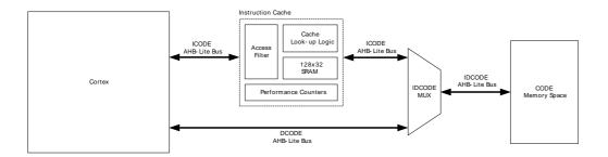
By default, the instruction cache is automatically invalidated when the contents of the flash is changed (i.e. written or erased). In many cases, however, the application only makes changes to data in the flash, not code. In this case, the automatic invalidate feature can be disabled by setting AIDIS in MSC\_READCTRL. The cache can (independent of the AIDIS setting) be manually invalidated by writing 1 to INVCACHE in MSC\_CMD.
