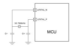
It is possible to connect an external clock source to HFXTAL\_N/LFXTAL\_N pin of the HFXO or LFXO oscillator. By configuring the HFXOMODE/LFXOMODE fields in CMU\_CTRL, the HFXO/LFXO can be bypassed.
