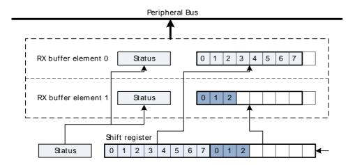
The two buffer elements can be read at the same time using the USARTn\_RXDOUBLE or USARTn\_RXDOUBLEX register. RXDATA0 then refers to buffer element 0 and RXDATA1 refers to buffer element 1.
