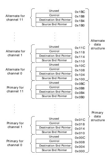
The controller uses the system memory to enable it to access two pointers and the control information that it requires for each channel. The following subsections will describe these 32-bit memory locations and how the controller calculates the DMA transfer address.
