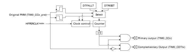
The DTI unit is enabled by setting DTEN in TIMERO\_DTCTRL. In addition to providing the complementary outputs, the DTI unit then also overrides the compare match outputs from the timer.
