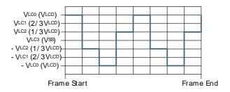
1/3 bias and duplex multiplexing - LCD\_SEG0-LCD\_COM0
