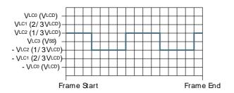
1/3 bias and quadruplex multiplexing - LCD\_SEG0-LCD\_COM2
