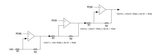
Table 30.5. Cascaded Inverting PGA Configuration
