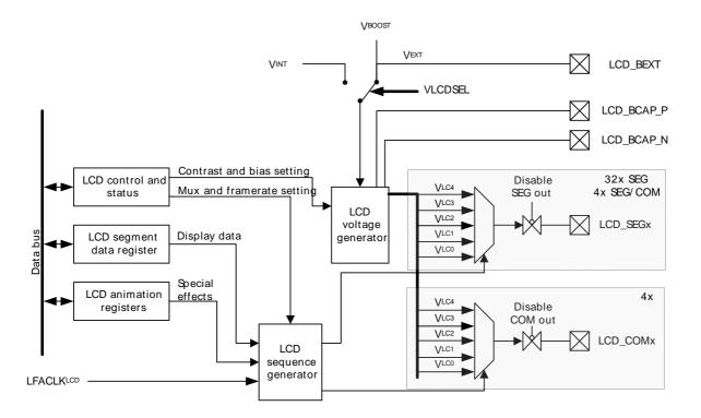
For simplicity, only one segment pin and one common terminal is shown in the figure.
