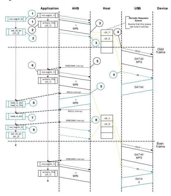
Interrupt Service Routine for Isochronous OUT Transactions in Slave Mode
