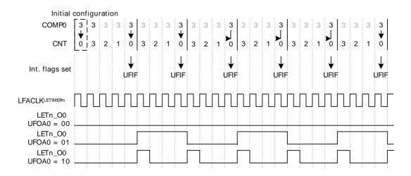
For the example in Figure 23.7 (p. 593), the One-shot repeat mode has been selected, and LETIMERn\_REP0 has been written to 3. The resulting behavior is pretty similar to that shown in Figure 6, but in this case, the timer stops after counting to zero LETIMERn\_REP0 times. By using LETIMERn REP0 the user has full control of the number of pulses/toggles generated on the output.
