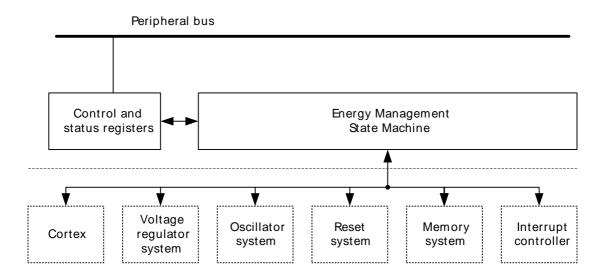
The EMU is available as a peripheral on the peripheral bus. The energy management state machine is triggered from the Cortex-M3 and controls the internal voltage regulators, oscillators, memories and interrupt systems in the low energy modes. Events from the interrupt or reset systems can in turn cause the energy management state machine to return to its active state. This is further described in the following sections.
