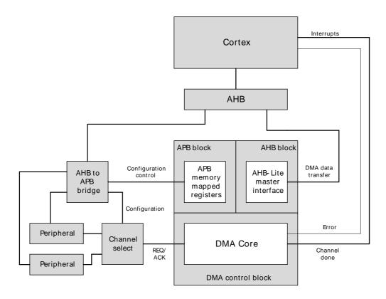
The DMA Controller consists of four main parts:
