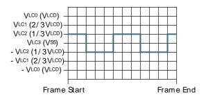
1/3 bias and triplex multiplexing - LCD\_SEG0-LCD\_COM1
