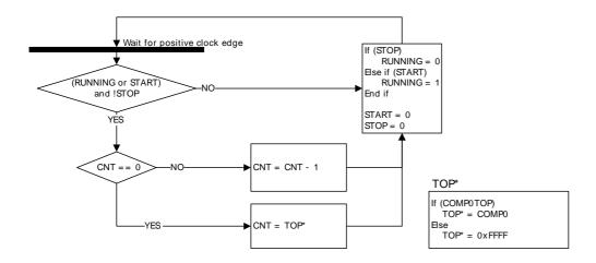
Note that the CLEAR command bit in LETIMERn\_CMD always has priority over other changes to LETIMERn\_CNT. When the clear command is used, LETIMERn\_CNT is set to 0 and an underflow event will not be generated when LETIMERn\_CNT wraps around to the top value or 0xFFFF. Since no underflow event is generated, no output action is performed. LETIMERn\_REP0, LETIMERn\_REP1, LETIMERn\_COMP0 and LETIMERn\_COMP1 are also left untouched.
