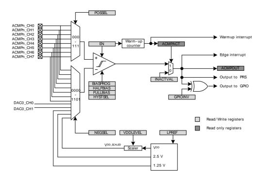
The comparator has two analog inputs, one positive and one negative. When the comparator is active, the output indicates which of the two input voltages is higher. When the voltage on the positive input is higher than the voltage on the negative input, the digital output is high and vice versa.
