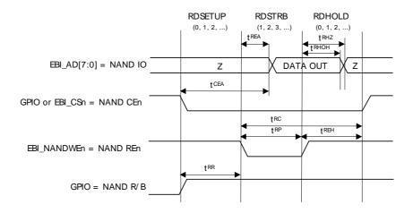
The EBI\_RDTIMING(n) setting requirements for satisfying the NAND Flash timing parameters for data output timing are shown in Table 14.6 (p. 196) .
