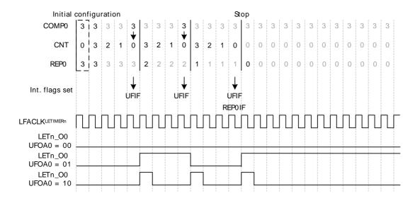
Using the Double repeat mode, output can be generated on both the LETIMER outputs. Figure 23.8 (p. 594) shows an example of this. UFOA0 and UFOA1 in LETIMERn\_CTRL are configured for pulse output and the outputs are configured for low idle polarity. As seen in the figure, the number written to the repeat registers determine the number of pulses generated on each of the outputs.
