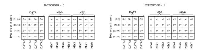
The registers DATA3-DATA0, are not memory mapped directly, but can be written/read by accessing AES\_DATA or AES\_XORDATA. The same applies for the key registers, KEY3-KEY0 which are
