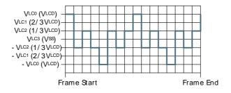
1/3 bias and quadruplex multiplexing - LCD\_SEG0-LCD\_COM1
