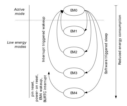
No direct transitions between EM1, EM2 or EM3 are available, as can also be seen from Figure 10.2 (p. 107) . Instead, a wakeup will transition back to EM0, in which software can enter any other low energy mode. An overview of the supported energy modes and the functionality available in each mode is shown in Table 10.1 (p. 108) . Most peripheral functionality indicated as "On" in a particular energy mode can also be turned off from software in order to save further energy.
