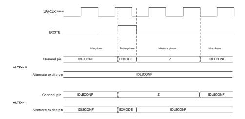
The alternative excite pins, LES\_ALTEXn, have the possibility to excite regardless of what channel is active. Setting AEXn in ALTEXCONF will make LES\_ALTEXn excite for all channels using alternative excitation, i.e. ALTEX in CHx\_INTERACT is set.
