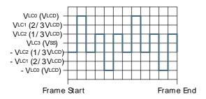
1/3 bias and triplex multiplexing - LCD\_SEG0-LCD\_COM2
