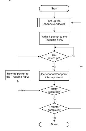
Figure 15.9. Receive Transaction-Level Operation in Slave Mode
