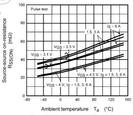
Fig. 10.6 R<sub>SS(ON)</sub> - T<sub>a</sub> (Note 6)
