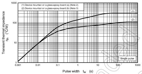
Fig. 10.12 r<sub>th</sub> - t<sub>w</sub> (Note 4) (Guaranteed Maximum)
