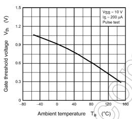
Fig. 10.9 V<sub>th</sub> - T<sub>a</sub> (Note 5)
