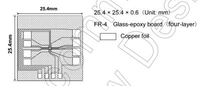
Fig. 5.2 Device Mounted on a Glass-Epoxy Board (b)
