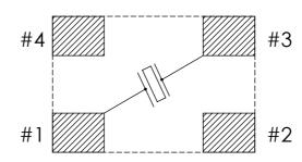
Do not design any conductive path between the pattern
