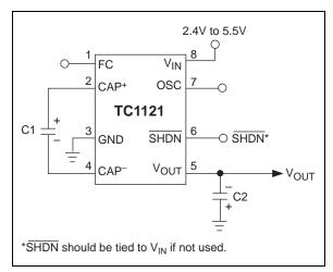
FIGURE 3-1: Charge Pump Inverter
