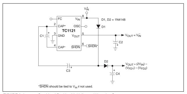
FIGURE 3-4: Combined Positive Multiplier and Negative Converter
