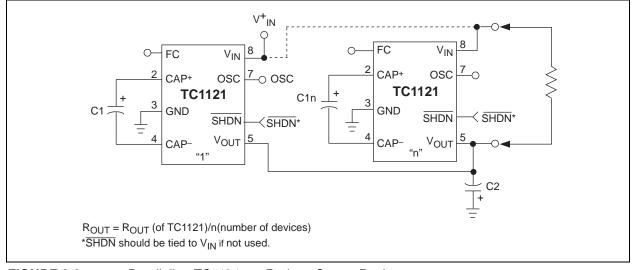
FIGURE 3-3: Paralleling TC1121s to Reduce Output Resistance
