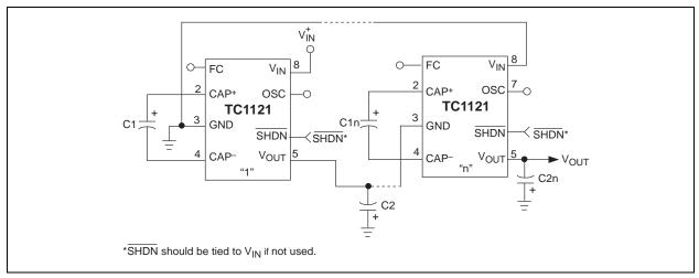
FIGURE 3-2: Cascading TC1121s to Increase Output Voltage
