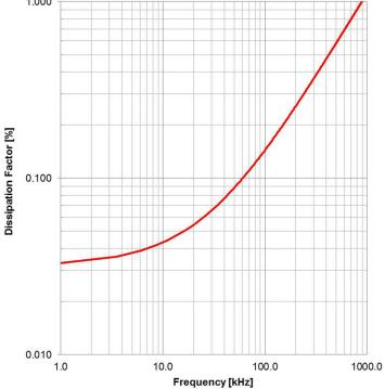
Test Equipment: E4991A or equivalent
